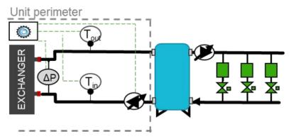
Bluethink solution for variable flow systems - ideal for systems featuring a primary and a secondary circuit physically divided by a heat exchanger or a tank with multiple connections.
