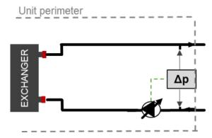
Flowzer VD requires two pressure transducers to be installed in the machine. Through these transducers, the inverter can gauge the actual pressure at the ends of the system and it can automatically adapt the pump speed to obtain a set available discharge head value. Flowzer VD must be combined with Flowzer VP. This accessory therefore allows a constant pressure system to be achieved.
